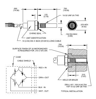
STANDARD TOLERANCE INCHES (MILLIMETERS) .XX = +/- .03 (.X = +/- .8) .XXX = +/- .010 (.XX = +/- .25)
